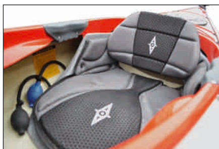
AIR seat including 4 Airbags in GTE versions of XO11 & XO13
